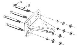
(4) The slots on the bracket allow small differences in alignment to be corrected. Fix the bracket with the nuts when the bracket is perfectly level. (Fig.5)
