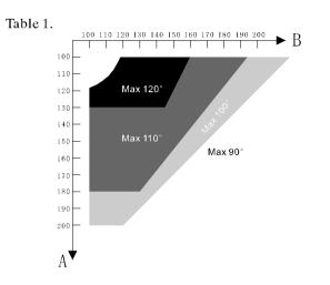
(3) Refer to Table 1 and choose the sizes of A and B in order to confirm the position where the rear brackets will be mounted. Use the bracket itself as a reference (Fig.4), mark the drill points for the rear bracket. Drill 4 holes (A) in the mounting surface, and fix the bracket with the appendant setscrews(B), then fix the bracket with screw nuts.
