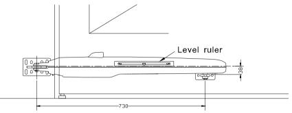
(6) Fix the front bracket to the leaf with a clamp provisionally (Fig.7). Lift up the gearmotor and fit the fork into the hole in the front bracket, keep the gearmotor lifted and pull it to open the gate until the hole in the bracket matches the hole in the gearmotor. Fix the gearmotor to the rear bracket with the cotter pin and then insert the clevis pin into the cotter pin. (Fig.8)
