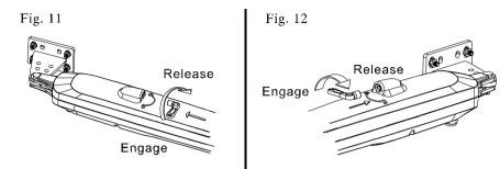
The clutch release for the left gearmotor The clutch release for the right gearmotor
