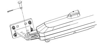
(7) Fix the gearmotor to the front bracket and anchor it with the appendant screws (D) and washers (C) with the gearmotor, fully tighten the screw. (Fig.9)
