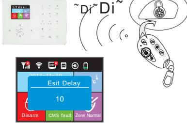
Press the arm key on remote or the keypad, then you hear system armed, please exit the protected area there will be tone to confirm the system is armed successfully.
