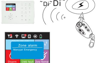
Press the panic button on remote, or press 3 key on panel for 3 seconds, it will trigger to alarm.
