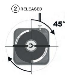
Remember to turn the MANUAL RELEASE knob back to position 1 LOCKED to restore the electric lock operation with mains power supply on.
