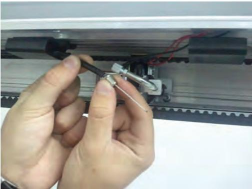
Fit the sheath end on the tip of the sheath which has been cut.
