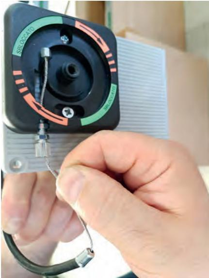
Insert the steel cable into the release handle and into the sheath until reaching the electric lock.
