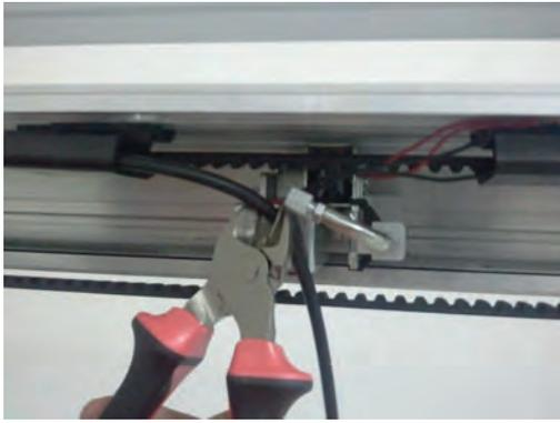
Insert the sheath using the cable guides until reaching the electric lock.
