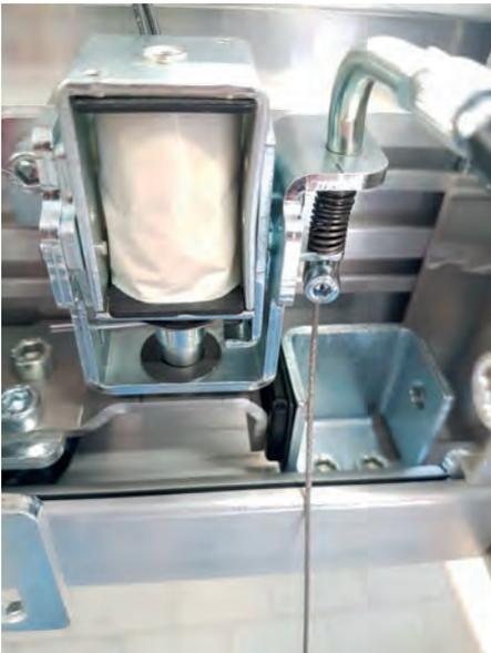
When the handle is in released position, the electric lock must remain open and release the leaves.
