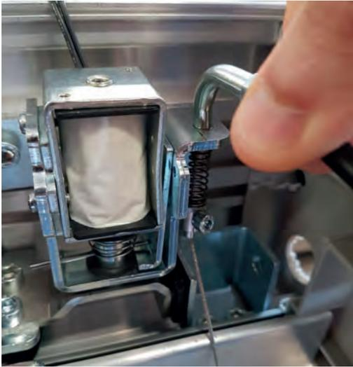
Check manual release operation, when the handle is in locked position, the electric lock must operate normally.
