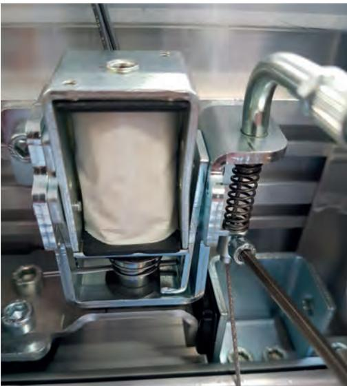
Position the compression spring and insert the metal cable inside the special release anchor, then lock it with the screw clamp.
